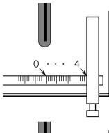
Feed the workpiece along the rip fence to cut in 4 cm.
