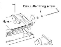
Remove the disk cutter fixing screw, turning counterclockwise with the hex key (long). Then, remove the disk cutter.
