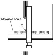
Move the rip fence so that its left edge contacts "4" graduation and secure tightly.
