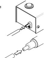
Install the appropriate nozzle and cup at the tip of the probe. When use the nozzle "fine", cups are unnecessary. Refer to the specifications in selecting nozzle type and cup The same of the sa size.
